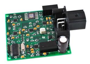
High precisión and high speed response 2D positioning sensor which gives an incident beam position in the (x,y) format. High results uniformity over the full sensor range. Extremely low dark current and large operation spectral range (400-1100nm). Includes an improved tetra-lateral Hamamatsu sensor for superior position detection.
